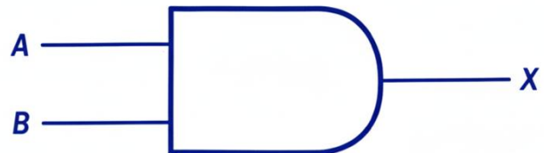
Simbol Gerbang AND – Gambar Ilustrasi Penerbit
